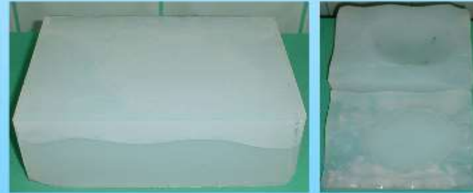
Vacuum casting of the silicone rubber moulds, made at DME - TUCN
