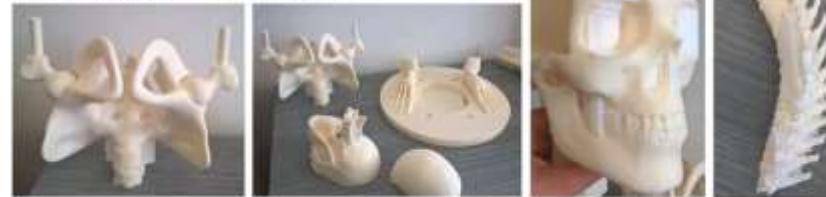
Fig. 9 Several parts of the skeleton model produced by FFF additive method
