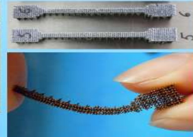
Samples made out of Ti based materials, with 0.6 mm hatching distance on X and Y
